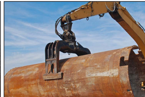
Grapple Arms Slip Into Sand Bucket & Hold In Place Via Gravity
