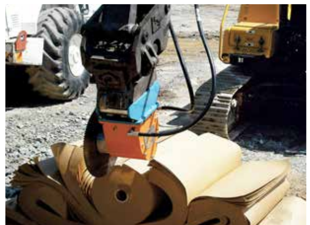
☛ Echidna rocksaw used for cutting paper rolls at a paper mill. (Visy, Australia)
