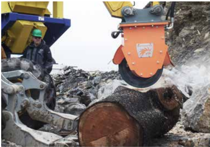
☛ Echidna Sg4 stump grinder demonstration. (Beluno, Italy)
