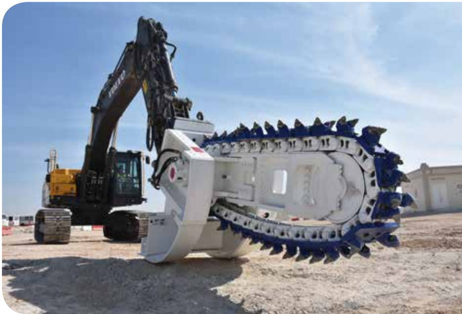
Qatar The new KEMROC trencher ETR 3 is a 60 cm wide and up to 2 m deep trench in medium hard limestone. The trencher is mounted on an EC 380 Volvo Excavator.
