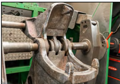
4 Freshly refurbished jaw
