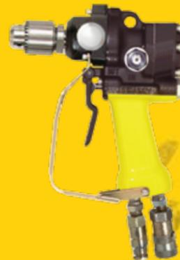
The DL07 is a variable speed drill with reverse capability. It features a 1/2 inch keyed chuck, dual position assist handle, dual-spool for open center or closed center operation, trigger guard, and is powered by an integral Hyrevz™ motor. A reverse-flow check valve prevents operation if tool is plumbed backwards. The DL07 is furnished with flush face quick disconnect couplers.
