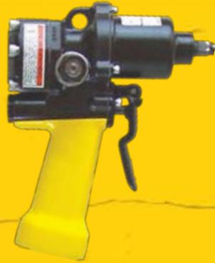
The ID07 is a high torque impact wrench used for tightening and loosening nuts and driving lag bolts. Delivers impact torque of up to 500 ft. lbs. / 675 Nm. Available with friction ring or pin type socket retainer.
