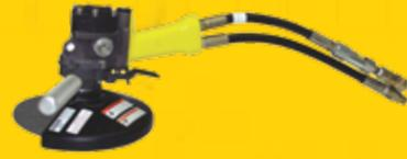
The GR30 can be used for grinding and cleaning with either cup or standard type grinding wheels and wire or nylon brushes. The GR30 features an assist handle, adjustable, rotating wheel guard, insulated handle, flow control for over-speed prevention, counter-clockwise rotation and is powered by an integral Stanley Hyrevz™ motor. The GR30 is furnished with hose whips and flush face quick disconnect couplers.
