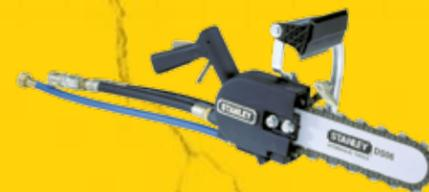
The DS06 is lightweight, powerful and ideal for fast cutting of concrete, reinforced concrete, conduit, brick, stone and other masonry. 13 inch plunge cut capability allows quick cutting of window, door, conduit and duct openings in walls and notching and trimming of concrete pipe. Trigger activated water for lubrication and cooling is ported through the bar and applied at the point where the concrete is being cut.
