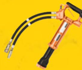
The CH18 is a light but powerful chipping hammer designed for medium duty chipping. It is commonly used for manhole and utility vault modifications or masonry repair and demolition. The tool's "D" handle and tool bit holder are shock and heat insulated for operator comfort. Tool steels are held in place by a slide that is ball-and-spring detented. The CH18 uses standard .580-inch hex, round collar, chipper tool bits and comes with hose whips and flush-face quick disconnect couplers.
