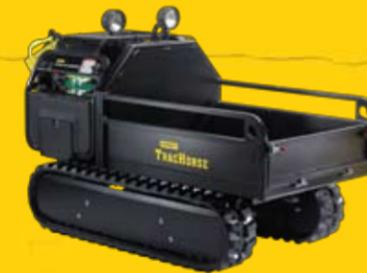
The TracHorse is an all-terrain, self-propelled mobile hydraulic tool and equipment carrier that allows transportation of tools and equipment in most job site environments. Simple operating controls allow for maneuvering in a wide range of applications. The auxiliary hydraulic tool circuit is designed for continuous-duty applications and features the standard high-efficiency cooling found on all Stanley hydraulic power units.
