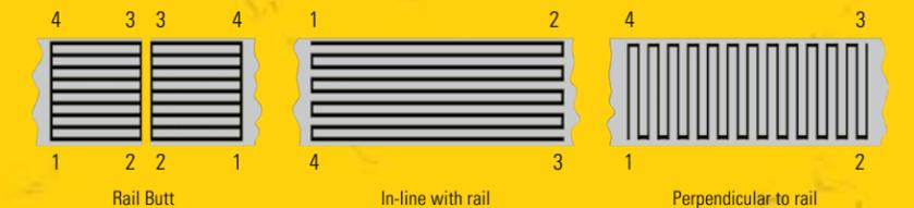
The following example shows a frog with 3 welding area selections. Each area was selected by pointing the weld tip at 4 points along the perimeter of each area.
